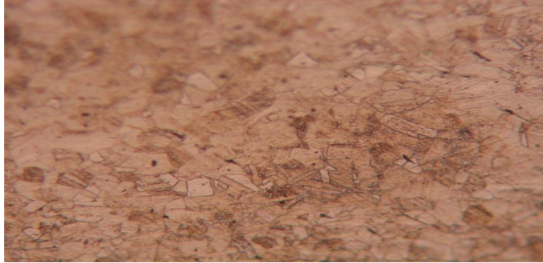
Figure 3: Microstructure of 316 Stainless steel (Electrolytically etched, 200X)
