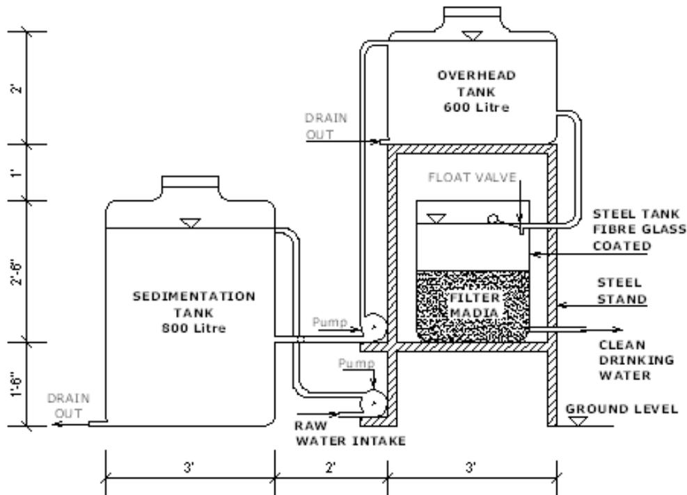
**Figure1:** Treatment Plant of 600 L/Hr Capacity
