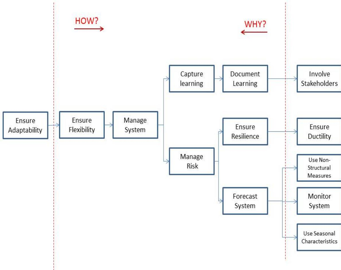
Figure 3. FAST diagram of Holistic Design of Adaptive Hydraulic Structures
