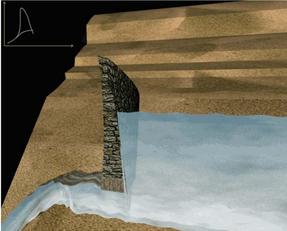
**Figure 4:** Flood Attenuation in Abbasi retarding Dam
