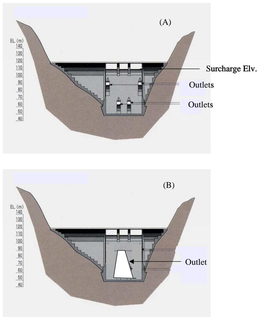
**Figure 8:** Modification of flood control dam
