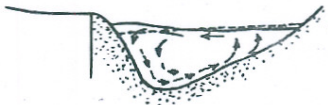
FORMATION OF A HOLE BY SCOUR
