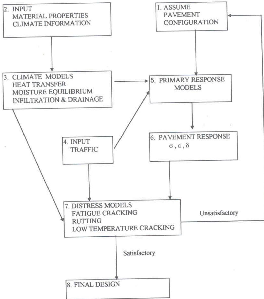
Figure 2. Schematic of the Mechanistic-empirical procedure.
